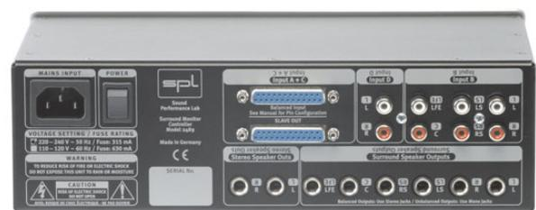
**I/Os:** Balanced 5.1 + stereo input (+4dB, Sub-D 25); unbalanced 5.1 + stereo input (0 dB, RCA); Sub-D 25 slave out; balanced 1/4" TRS surround and stereo speaker outputs.
