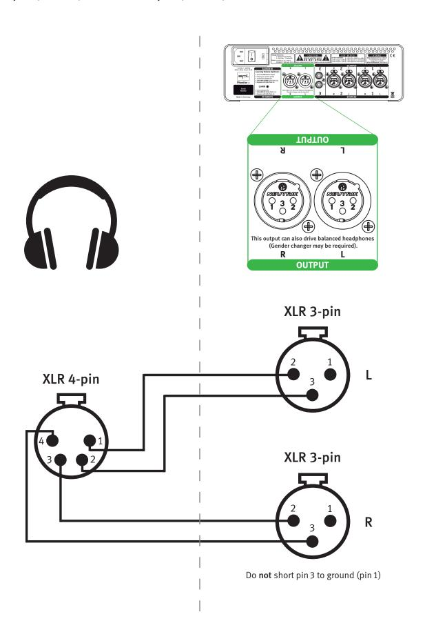
Balanced headphones with **two 3-pin XLR plugs** can be connected to the Phonitor2 with **two female/female gender changers**.
