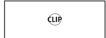
At all relevant points of the signal flow the display gets read off: behind the Pre-amplifier, behind the Compressor/Limiter, behind the EQ and behind the Output control. All possible causes for overload can be directly checked (overdriven Microphone/Instrument/Line Gain, an excessive Make Up value in the Compressor/Limiter, too much boost in the EQs or too high output level).
