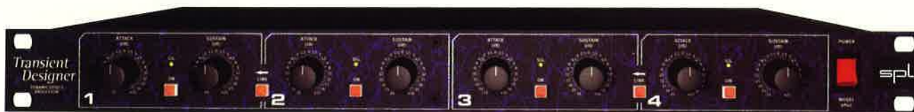
FIG. 1: The Transient Designer 4 uses VCAs controlled by envelope generators to process dynamics independent of levels.
