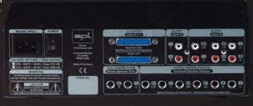
Balanced inputs A and C are on a single 25-pin Sub-D female with the usual Tascam pin-outs. Similarly the slave output is balanced and also uses a 25-pin female Sub-D. Inputs B and D are unbalanced phonos. All the speaker outputs are 1/4-inch jacks. Powering is built-in and there is a mains switch with a well subdued switch-on thump - unlike many of the more expensive units.
