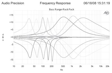
The diagram shows the different filter characteristics. The lower bands have relatively narrow bandwidths for fundamental tones. The upper bands have broader bandwidths to process groups of overtones in common.
