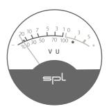
If the VU meters light up red permanently, the protection circuit has been activated. The output connectors are disconnected from the amplifier via a relay to protect the connected headphones. Please contact your local dealer for repair service.
