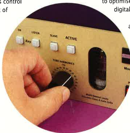
The Tube Harmonics control adds valve distortion products without increasing the overall signal level, so you can easily hear how the sound is really changing.
