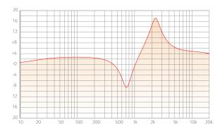
In position 6 (Ext) the external side-chain insert is activated. Via insert send and insert return, an external stereo equalizer can be integrated into the side-chain signal. Individual filter curves can be created to focus the response of the compression to certain frequency ranges.
