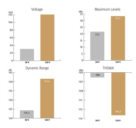
When it comes to volume, the 120V technology exhibits a performance that is twice that of common components and circuits, in regard to maximum level and dynamic range, with values that are approximately 10 dB higher. THD measurements of the the 120V technology more than 8 dB better than a device with a operating voltage of 30V.
