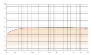
The next switch positions can be used to switch more complex filters into the side-chain signal. These can be used to focus the response of the compression to certain frequency ranges. This is also referred to as frequency selective compression.
