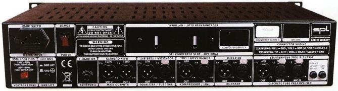
The Frontliner has balanced inputs and outputs for each processor that forms the recording channel.
