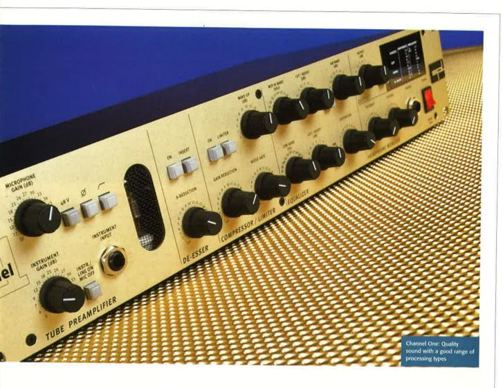
homes in on the narrow band of 's' frequencies and feeds a phase-inverted version back into the signal path, thus cancelling out any sibilant sounds while leaving adjacent frequencies untouched. An autothreshold is also featured, allowing constant de-essing regardless of input level.
