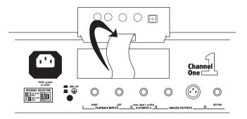
**Step 4:** Without turning it, insert the module into the device (circuit board upwards) and fasten it using the screws from the optional slot cover.
