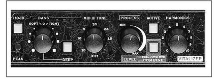
If you are working with a VITALIZER filter network for the very first time, it is advisable to operate the control parameters in a certain order to achieve optimum results as quickly as possible. You should use a mono signal of good quality as a signal source. You can either preamplify it in the INPUT section or feed it directly into the INSERT RETURN, so that the signal goes directly into the PARAMETRIC section.
