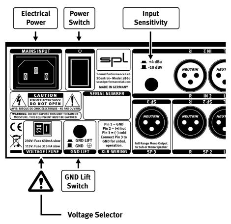
The rear panel VOLTAGE SELECTOR serves to let you switch to the local line voltage standard (115 V position: 110-120 volts/60 Hz, 230 V position: 220-240 volts/50 Hz). The diagram above shows the correct switch position for 230 V power supply.
