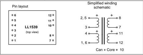
Spacing between pins: 5.08 mm (0.2") Spacing between rows of pins: 35.56 mm (1.4") Weight: 130 g
